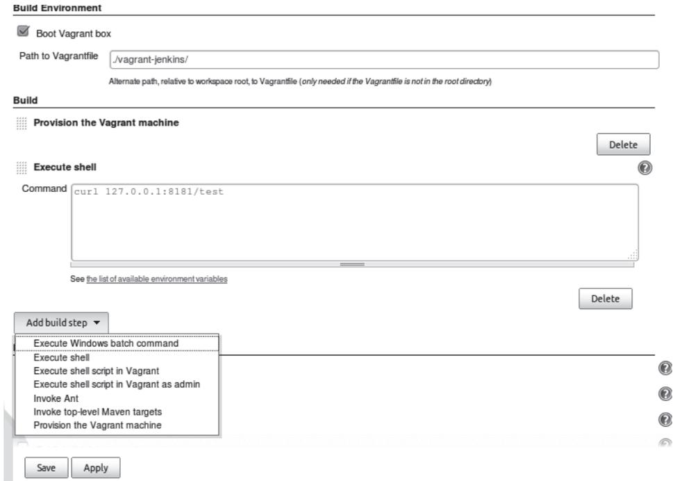
**Figure 9-2.** Configuration of Vagrant as Jenkins Build Job
